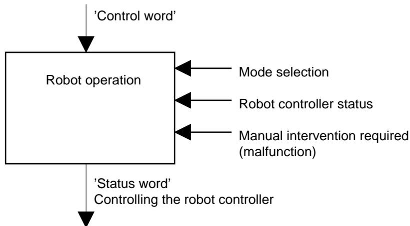
**Figure 5: Device control (robot operation) function block**
